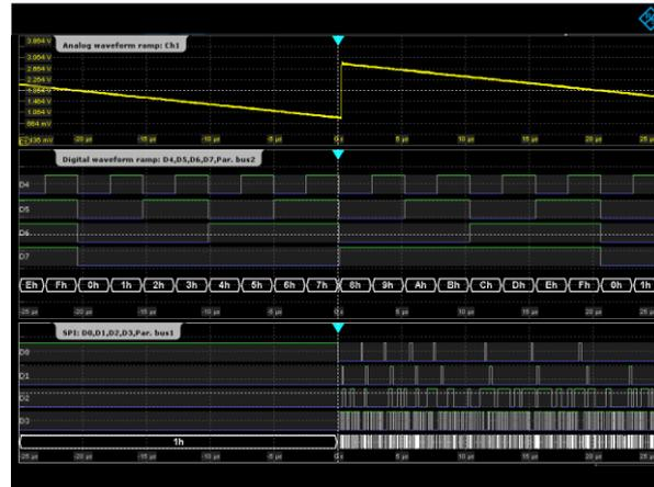
With the R&S®RTE-B1 option, every R&S®RTE can be turned into a mixed signal oscilloscope with 16 digital channels. This example shows the ramp signal of a 4-bit ADC with analog and digital channels correlated to an SPI bus that controls the ADC.
