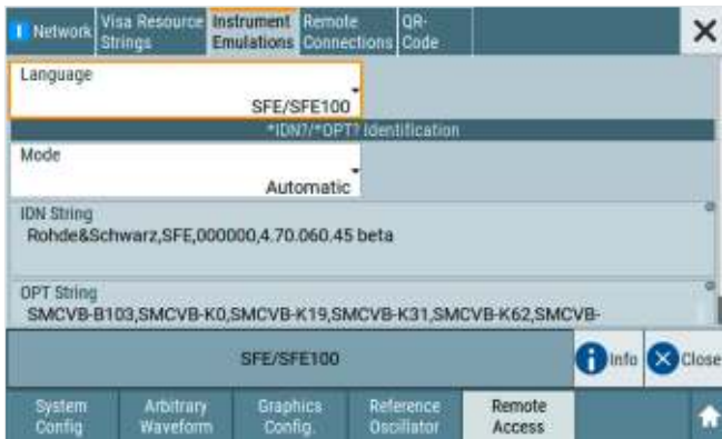
R&S®SMCV100B instrument setup for R&S®SFE100 emulation and replacement
