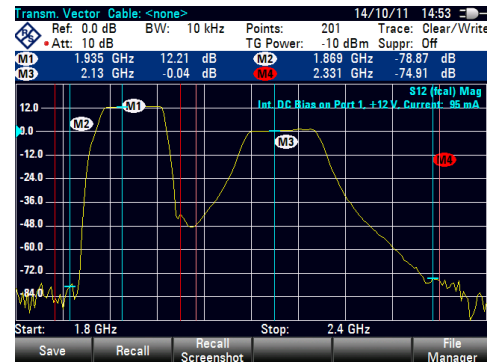
Two-port capability for transmission measurements. DC Bias
