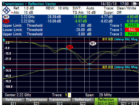
Simultaneous display of four S-parameters (S11, S21, S12, S22).
